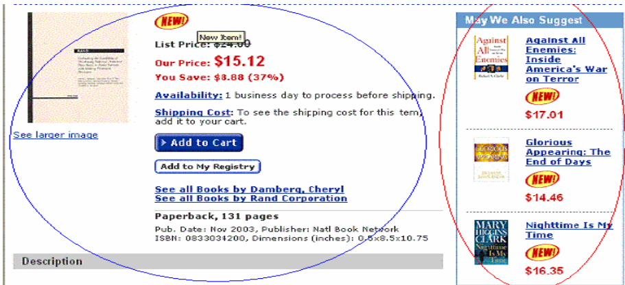
Fig. 2. It is a part of a web page taken from amazon.com. It shows disadvantage of fan-out approach for filtering noisy data. The region in left ellipse is actual data. Right ellipse contains secondary data. Since the fan-out of data in left ellipse is very small, it will get filtered with the above described approach
